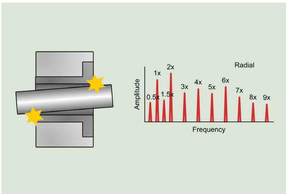
As the wear increases, the frequency spectrum changes, allowing a classification of the severity of the looseness into the following four groups:
