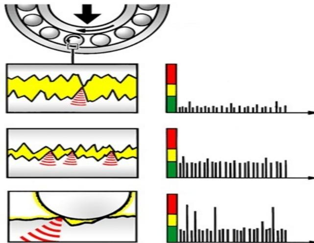
There are three condition zones namely Green for Good Condition, Yellow for Caution and Red for Damaged condition. The peak value measured by the operator gives the status of the machine and the zone it belongs to.
