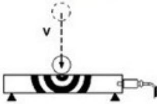
Event 1: a shock wave spreads through the material
